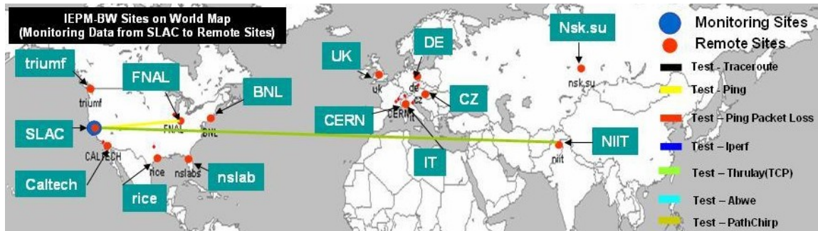
Figure 7 Deployment of the IEPM-BW hosts monitored from SLAC. The monitoring site (SLAC) is shown in blue, and the monitored sites in red. The colored lines indicates the test being made when the screen snapshot was taken
